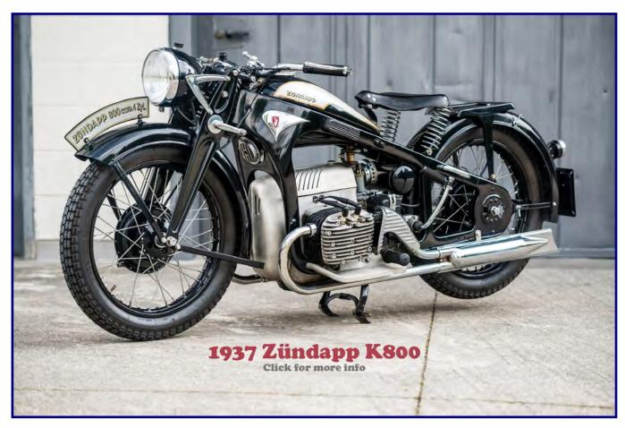
800cc Opposed 4 Cylinder 26 hp Flathead Engine. Shaft drive with 4 speed chain transmission, hand shift lever on right side. Left floorboard swings out to serve as side stand (some bikes).
